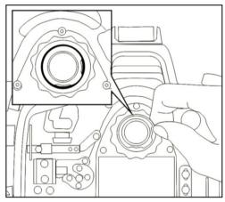
Remove the O-ring of the 0.66x viewfinder inside the rear half of the housing by making use of the recess on the viewfinder.
