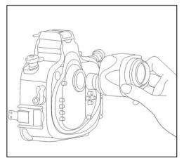
Align the viewfinder with the sleeve in the display window as shown in the diagram.
